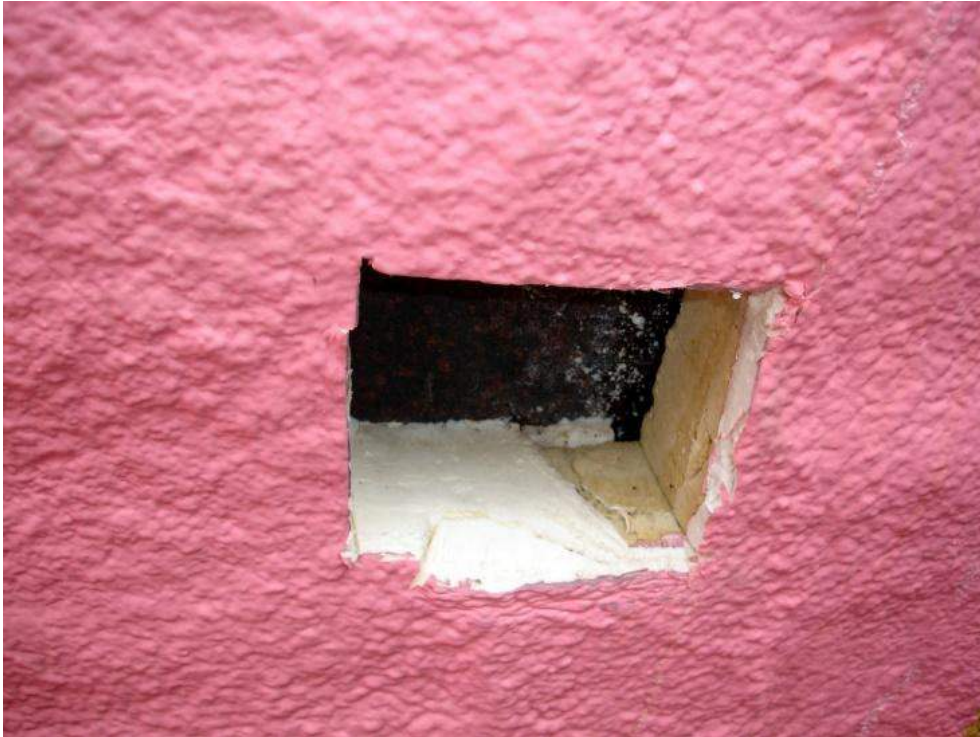
Figure 13. Test cut out to see how much “old” and “new” PU foam are reacting with each other and the underlying steel of the pipe
